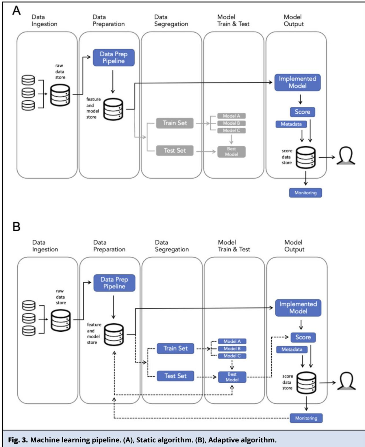
**Fig. 3. Machine learning pipeline. (A), Static algorithm. (B), Adaptive algorithm.**
